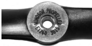
Most Master Airscrew Propellers have two hole sizes because they are piloted in the back of the propeller to facilitate reaming should you need to enlarge the hole. The first number is the hole size; second number is the pilot size.
