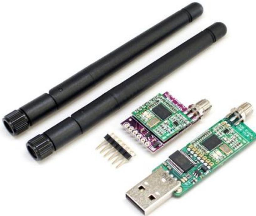
The 3DR Radios can connect to the FTDI /S0 port or to S3 on the S1-S3 port. I would recommend using the Rx3 and Tx3 on the S1-S3 Port, as this will leave the FTDI port free for other uses such as Bluetooth. Using the S3 port will also not require any baud rate changes in APM\_Config.h.
